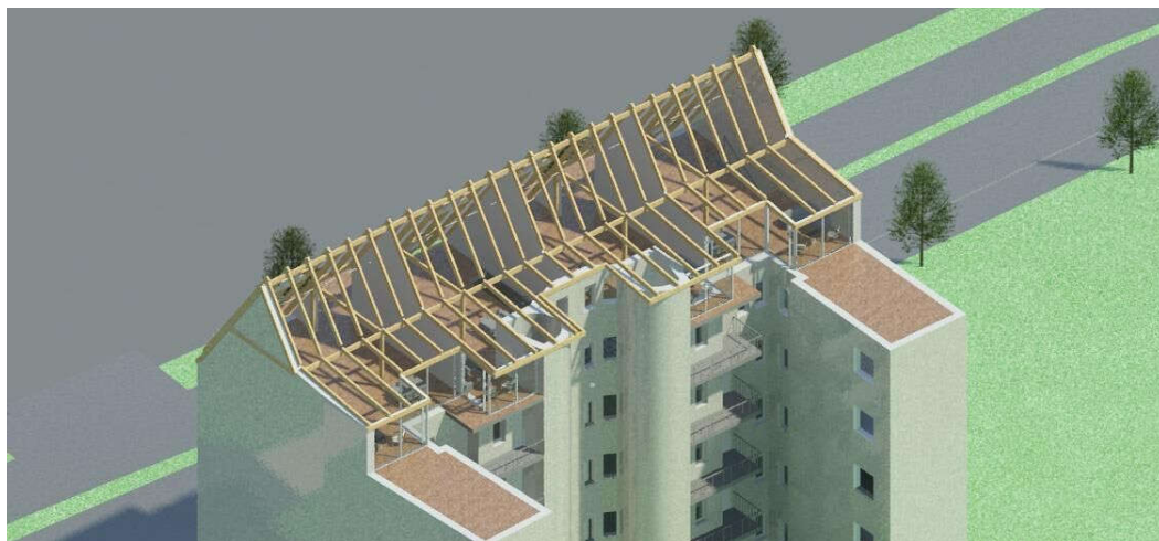
Figure 3 - Our carrying beam system
